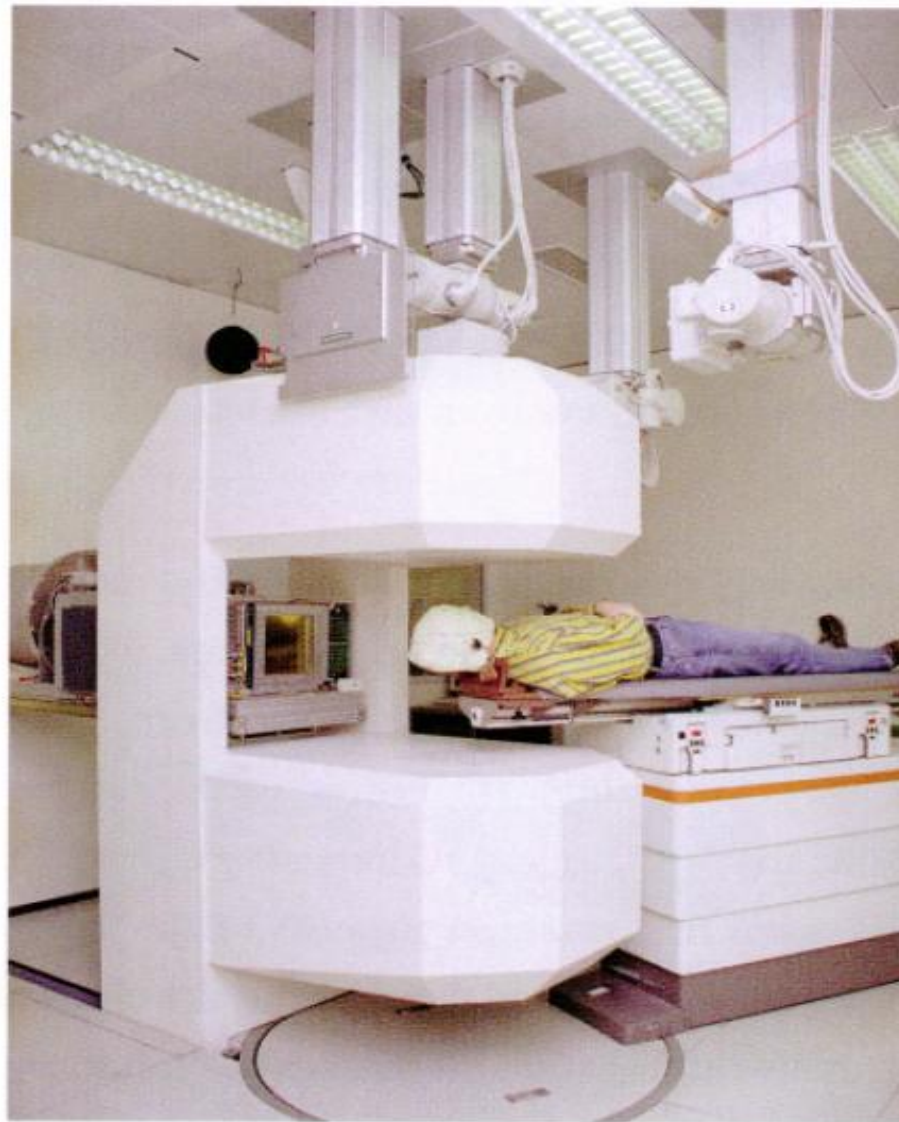
Fig.12: Patient positioned in front of the exit-window before irradiation. The X-ray equipment is removed and positioned at the ceiling. The two heads of the PET-camera are above and below the patient's head.
