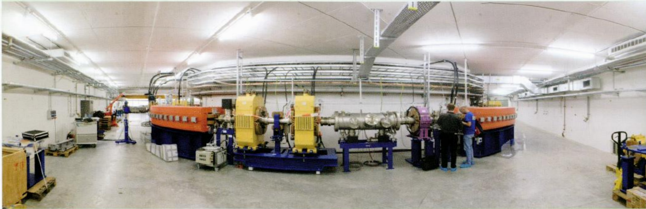
View of the accelerating synchrotron. Dipole magnets (in red) at the left and right held the beam on its duty cycle while the quadrupoles (yellow) focus the beam.
