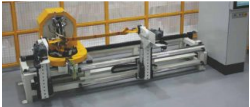
▲ New advanced NCT narrow coil taping machine from Ridgway
