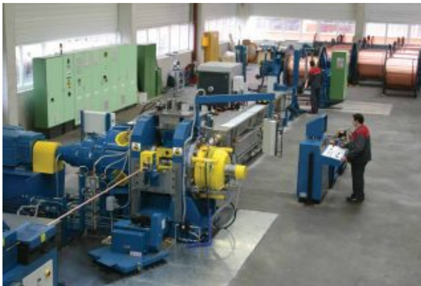
▲ A typical BWE Conform 550i installation for copper bus bar and sections
