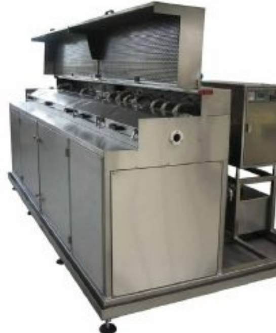
▼ The ultrasonic wire and strip cleaning system
