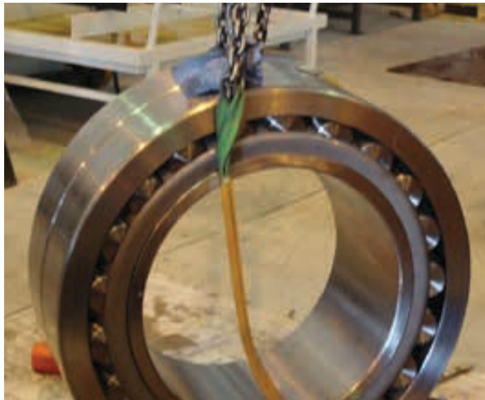
Above: Bearing remanufacture is possible in over 50% of cases and can normally be carried out within days at considerably lower costs compared to a new replacement. Left: SKF bearing designs are highly specialised to meet demanding conditions. Shown here is a remanufactured bearing being assembled.
