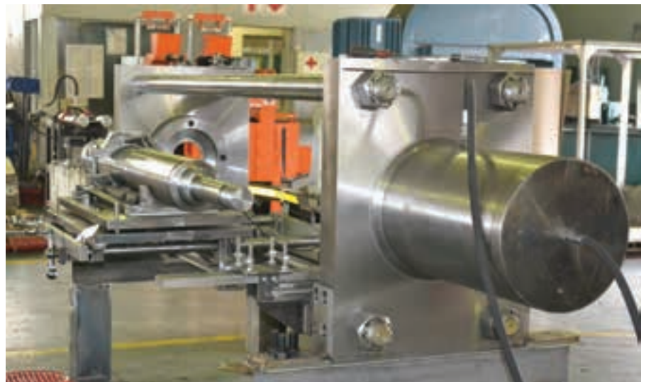
Under test at RBES' Jet Park premises is a custom built hydraulic press for manufacturing railway couplings.
