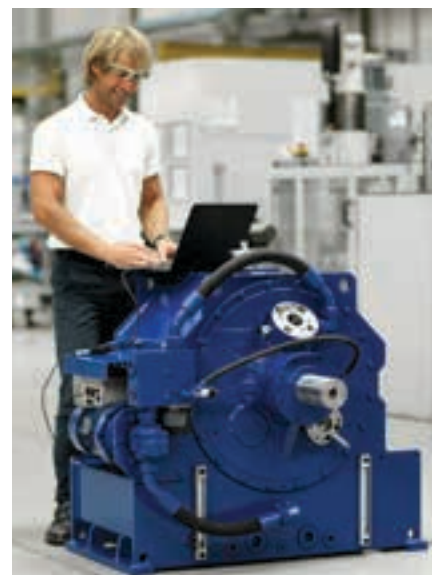
The Voith TurboBelt 500 TPXL comes with an integrated controller and offers condition monitoring as well as remote access.
