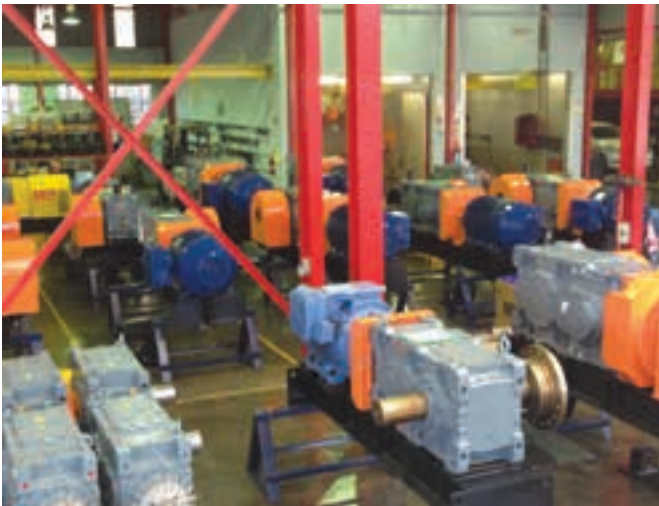
Left: According to Blickle, the bulk of SEW-Eurodrive's regional turnover is still generated by the mining and minerals-processing industry. Shown here are the company's X series helical and bevel helical gear units at the Johannesburg assembly facility. Right: A cement plant in Zambia supplied by SEW-Eurodrive with geared motor solutions.
