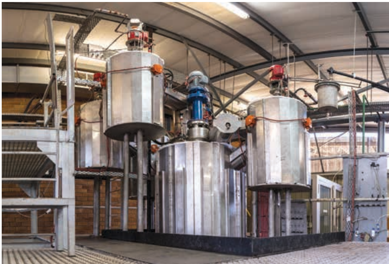
The CSIR's Titanium Pilot Plant, which produces titanium directly from titanium tetrachloride (TiCl 4 ) feedstock. This is reacted with a strongly reducing metal such as magnesium, sodium, calcium or lithium to remove the chloride and to give titanium powder and a salt.
