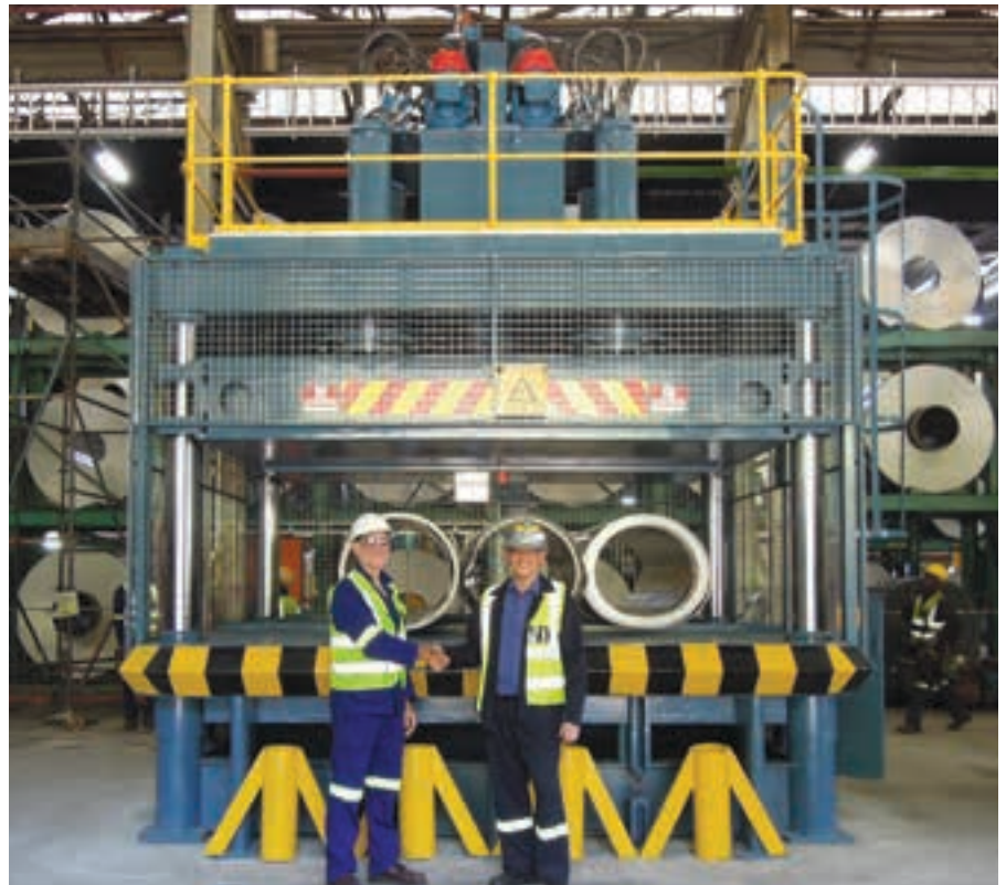
The pup-coil press built for Hualamin Aluminium uses a control strategy for a four-cylinder hydraulic press that always ensures the press remains parallel.
