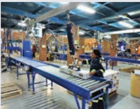
The end of a production line, where the JumboFlex vacuum tube lifter is used for palletising boxes of the RocLoc® resin capsules.
