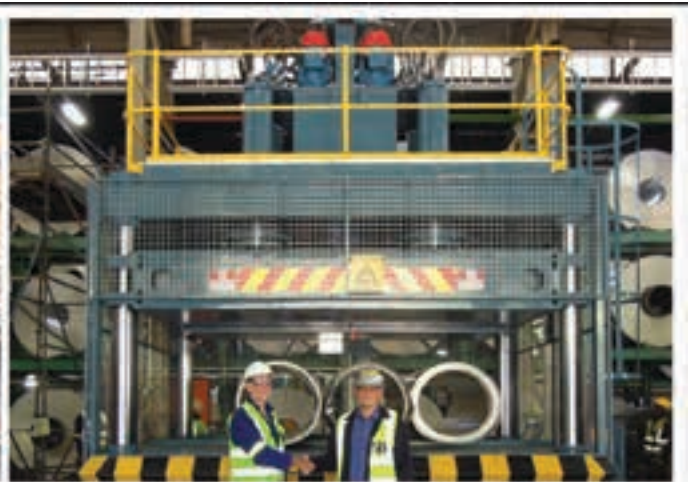
Press with unique self-leveling controls for even pressing of uneven materials, Hulamin Aluminum.
