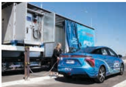
Toyota Australia's mobile hydrogen refueller incorporates a generator and a compressor mounted in a purpose-built trailer attached to a Hino 700-series truck.
