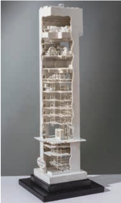
Printed using a ceramic material, the first 3D printed model produced by Murray & Roberts Cementation is of Ivanplats’ Platreef Shaft 2 headframe.
