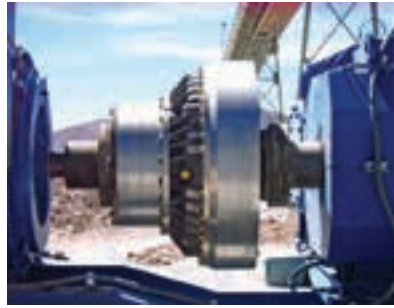
The Voith TVVS fluid coupling is predominantly used on belt conveyor drives for the mining and materials handling sectors.
