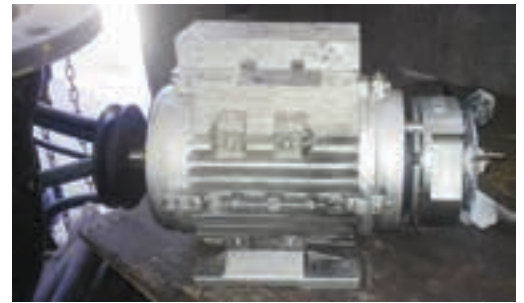
Bauer aluminium motors are far more lightweight than cast iron equivalents.
