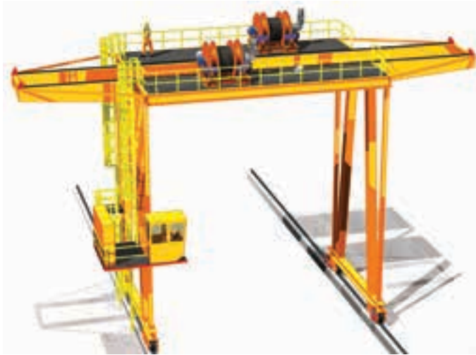
An illustration of the gantry: The stage is suspended from the gantry on steel wire ropes attached to two 8.0 t stage winders mounted on purpose-built platforms to the sides of main girders in double fall.
