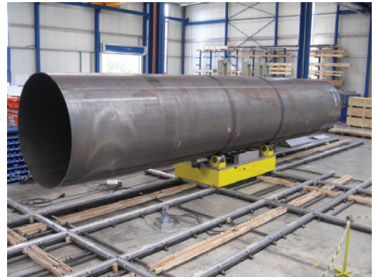
Transport track with crossing element, which allows for quick changes of travel direction
