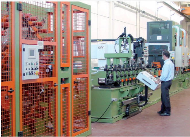
Stainless steel tube mill with LASER welding system and complete with vertical strip accumulator - max. production speed 20 m/min
