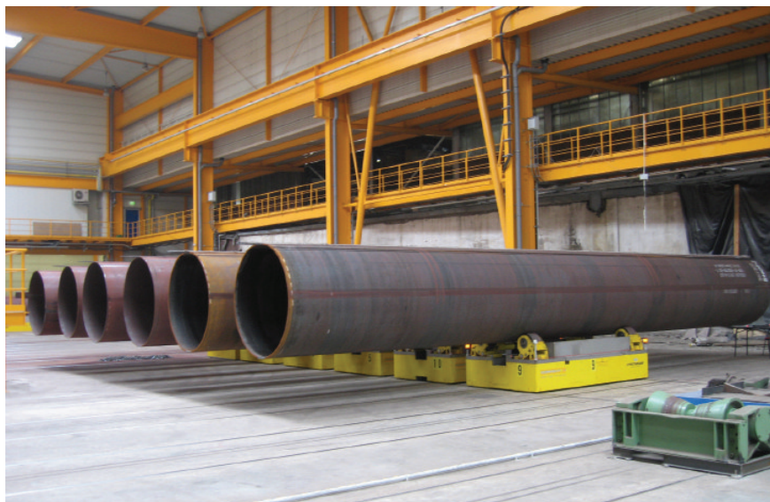
Bergrohr's new RoundTrack-based production facility, which transports large pipes weighing up to 30t
