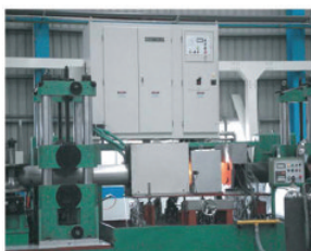
24" Pipe Mill And Annealing
