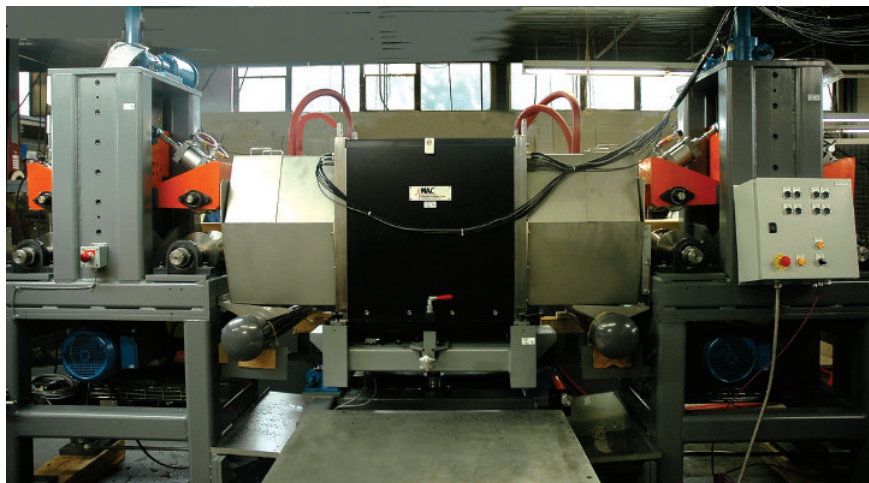
Magnetic Analysis Corp's Echomac® ultrasonic rotary inspection system designed for 220mm diameter tube. Pinch stands are used for driving and accurately positioning the tube are on either side of the UT rotary
