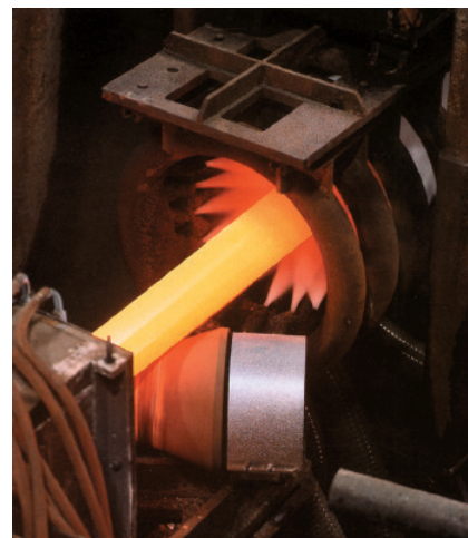
↑ Heating a pipe using machinery from Ajax Tocco
