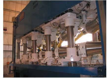
ⓘ A 10-roll straightening installation from Bronx/Taylor-Wilson
