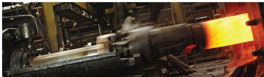
VVT's pipe is manufactured on 2 rolling mills: big and small Mannesmann pilger mills
