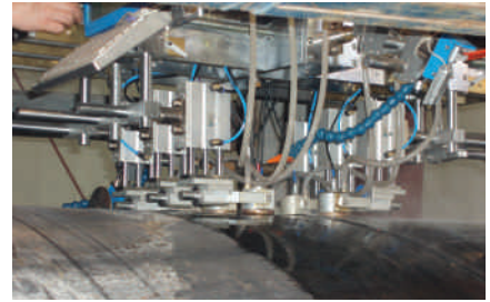
ⓘ Online weld examination
