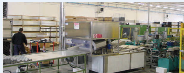
Figure 11-12: Automatic equipment (outer and inner) for ultrasonic cleaning, rinsing and drying of aluminium tubes for fumes discharge of house heating plant (productivity of 1 tube every 30 seconds)
