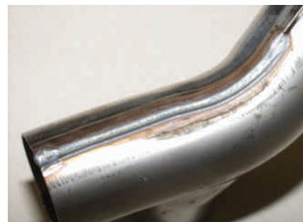
The almost spatter-free welds achieved by the cold process bridge high gap widths
