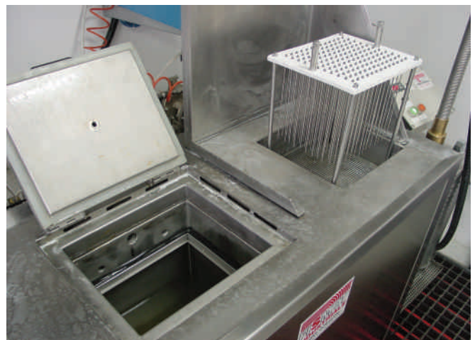
Figure 6: Cleaning equipment (inner and outer) for ultrasonic washing, rinsing and drying of stainless steel medical cannulae
