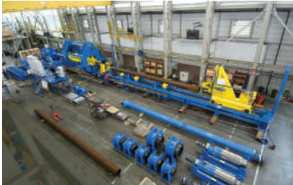
A pipe expander including new straightener, expander heads, draw bar for larger diameters and several toolsets
