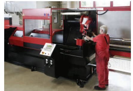
ⓘ Either HSS or carbide blades can be used, and a saw blade change takes approximately one minute
