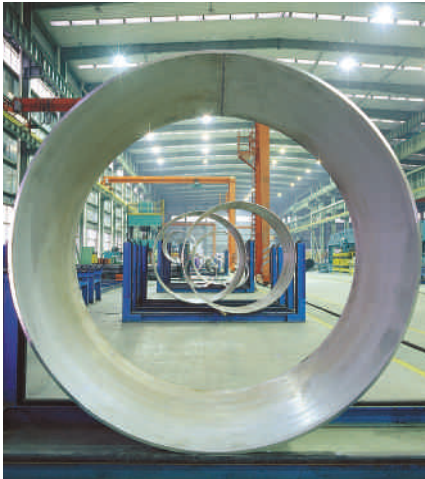
① Jiuli manufactures seamless tube from 6-273mm OD and welded tube from 9.53mm to 2,540mm OD
