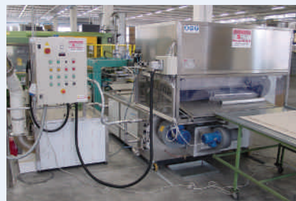
Figure 11-12: Automatic equipment (outer and inner) for ultrasonic cleaning, rinsing and drying of aluminium tubes for fumes discharge of house heating plant (productivity of 1 tube every 30 seconds)
