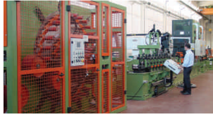
A stainless steel tube mill with laser welding system
