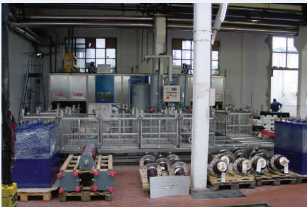
Figure 16: Automatic equipment (outer and inner) for ultrasonic cleaning, rinsing, and drying of ceramic insulators
