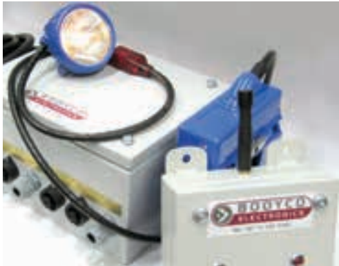
The mineworker is equipped with a two-way Radio Frequency Identification (RFID) tag fitted into a cap lamp cover that flashes a warning whenever he or she approaches machinery.
