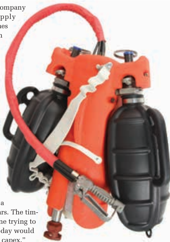
BME's reef-pump is light and small and easy to move around narrow stopes.
