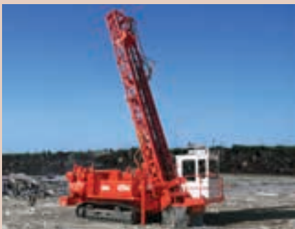
The Sandvik D25KS is a diesel-powered, self-propelled crawler-mounted blasthole drill rig.
