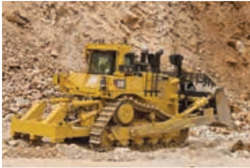
The Cat D10T2's mainframes are built to absorb high impact shock loads and twisting forces encountered during severe dozing and ripping applications.
