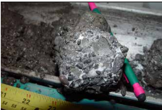
Figure 2.5: The Mallik site in Canada's Arctic. This has been the site of dedicated gas hydrate programs since 1998. The map (above) shows the route of the temporary ice road (red line) that provides access to the site near the shore of the Mackenzie delta. The photo (below) shows a sample of gas-hydrate-bearing coarse-grained sandstone recovered from the site in 1998. (Courtesy: Geological Survey of Canada.)
