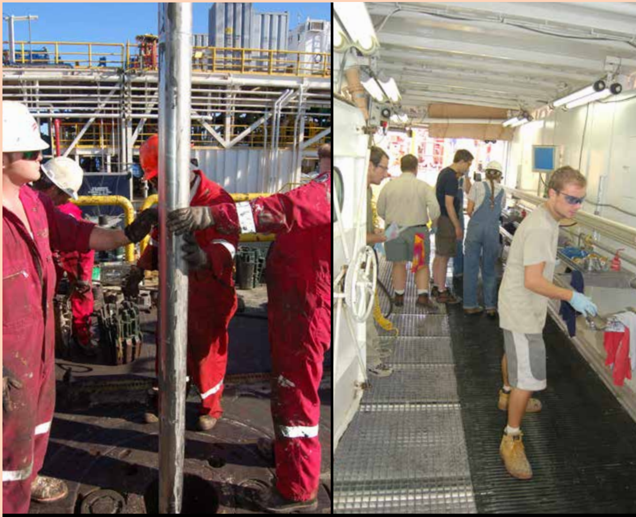
Figure TB-2.2: Gas hydrate evaluation. Left: Advanced well logging devices being deployed in the deepwater Gulf of Mexico (courtesy Gulf of Mexico gas Hydrate JIP Leg II Science Team). Right: Core samples are prepared for evaluation on the catwalk of the drill ship Joides Resolution, Bay of Bengal, India, in 2006 (courtesy NGHP Expedition-01 Science Team).
