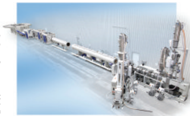
ⓘ KraussMaffei Berstorff supplied this complete extrusion line for PVC foam-core pipe
