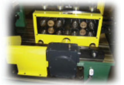
Figure 3 – Powered hemming unit with spur gears
