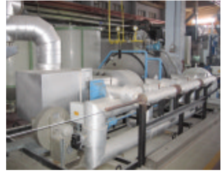
Figure 2: Universal's hot air dryer/thermal oxidizing system
