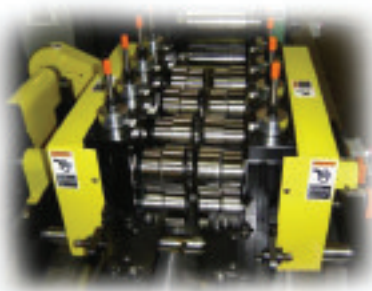
Figure 2 – Adjustable width hemming unit with digital indicators
