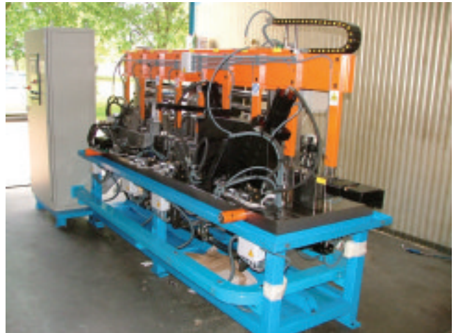
Menegon's automotive production line for cutting, shearing and folding
