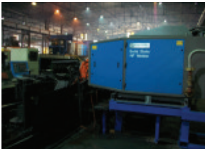
One of the CFI solid-state HF welders installed at Cayirova Boru
