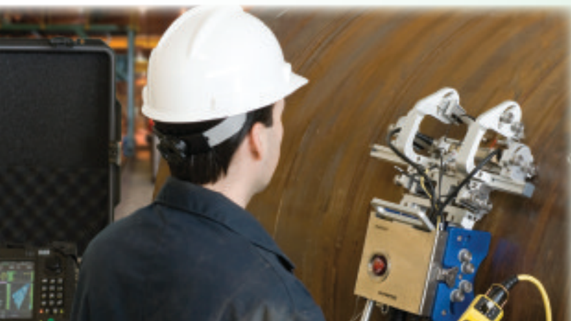
➤ The WeldRover™ automated scanner for NDT testing (NDT) on pipe (see page 109)
