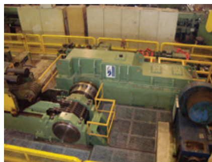
Gear reducer for drawing tubes in production at the facility in Marcegaglia, Boltiere, Italy
