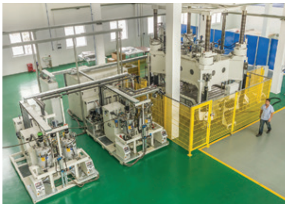
The RimStar Compact 8/4 RTM and RimStar Compact 8/8 RTM metering machines
