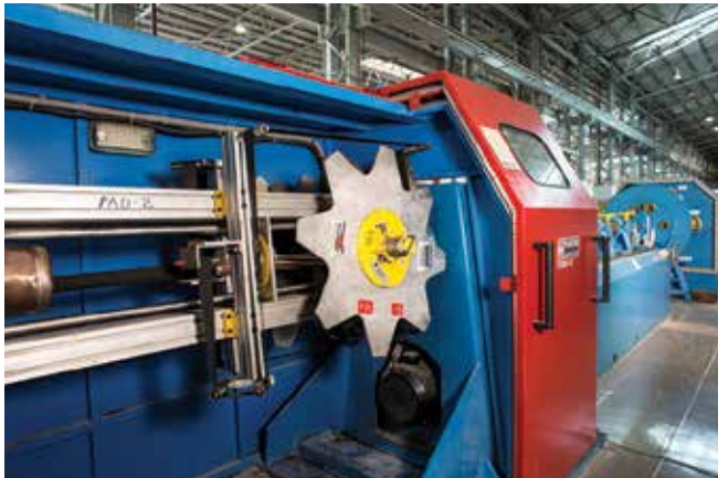
▲ A high-speed tangential taping head from Pourtier
