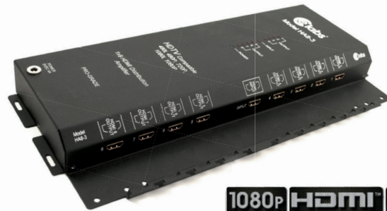
HA8* 1 In / 8 Out HDMI 1.3 A/V Distribution Amplifier Commercial grade & capable of 1080p @ 60Hz, the HA8 1 x 8 High Definition Distribution Amplifier distributes one high definition source to multiple displays.
