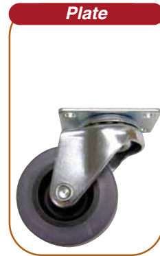
Top Plate w/Brake Top Plate Size 1-3/16" x 2" spacing 13/16" x 1-9/16" 3/16" diameter bolt
