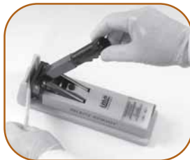
Lift handle and insert pouch either from the top or the sides between the crushing plates.
