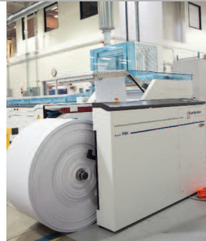
Darwill recently added a Hunkeler RW6 Rewinder to its second Roll-to-Stack line, which now has the capability to also go roll-to-roll.
