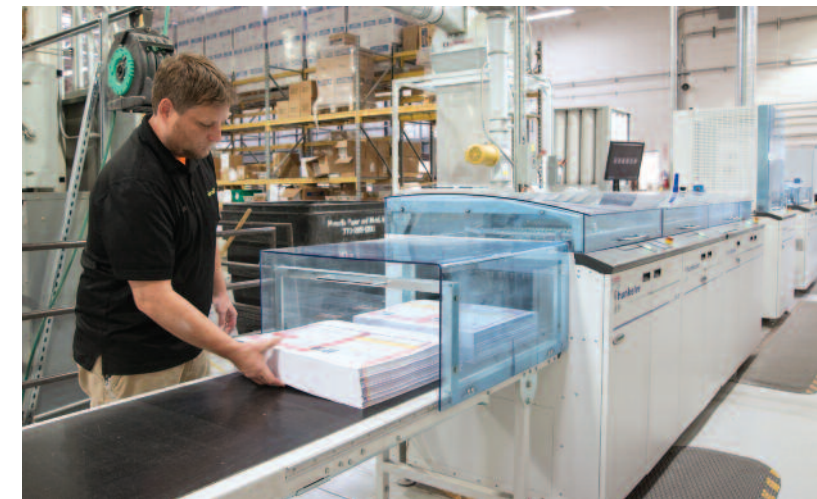
Bob VanWinkle operates the Canon ColorStream press with in-line Hunkeler Roll-to-Stack solution and DP6 Dynamic Perforator.
