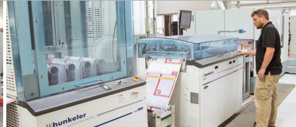
Darwill recently added a Hunkeler RW6 Rewinder to its second Roll-to-Stack line, which now has the capability to also go roll-to-roll.
