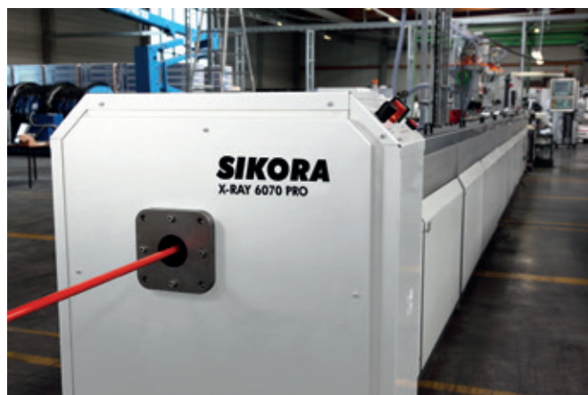
Figure 4: X-ray measuring system installed in a hose extrusion line
