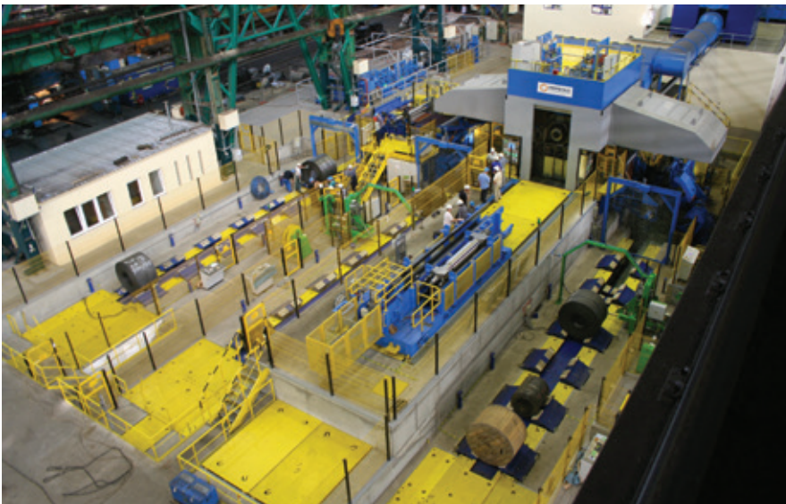
Reversing cold mill from Primetals Technologies. A comparable mill will be installed in the Ixtaczoquitlan production plant of Tyasa
