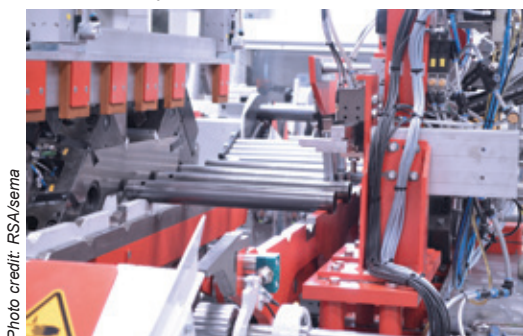
Double-side punching of up to eight holes simultaneously
