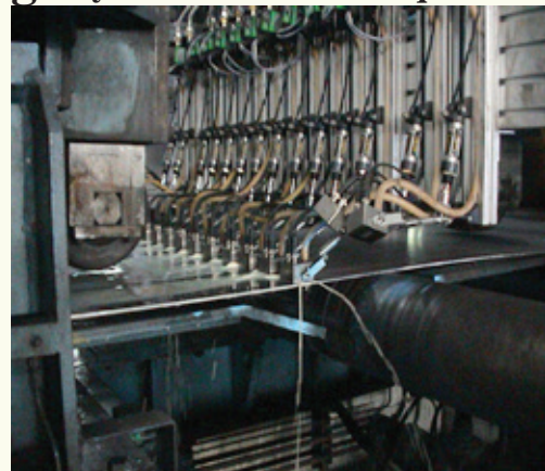
ERW mill 1900 mm coil - Thickness 4-16 mm
