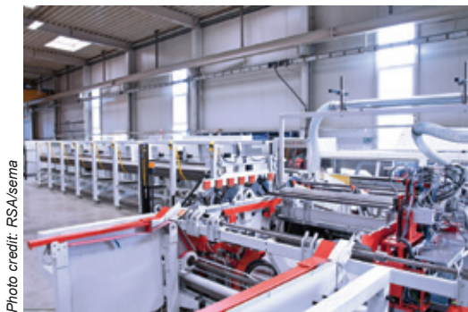
Double-side punching of up to eight holes simultaneously
