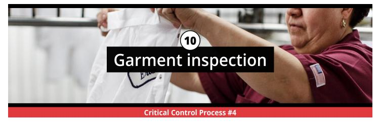
Clean garments are removed for the garment cart and placed on a hanger. During this process the operator visually inspects the clean garment per the Corporate- Garment Quality Specifications. If the clean garment does not meet the Corporate- Garment Quality Specifications the garments RFID chip is scanned into the mending RFID antenna, placed on the steam tunnel conveyor, travels through the steam tunnel and drops off the conveyor to the garment mending area.
