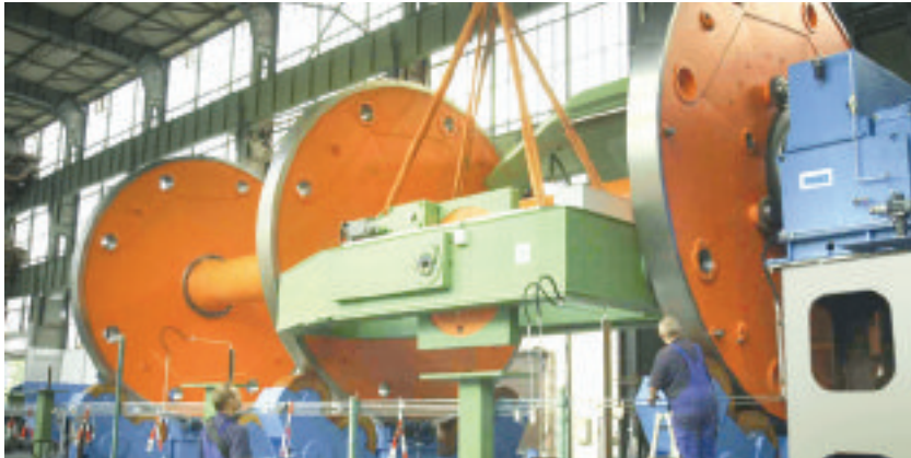
▲ A closing cage type MKVS 8x2700 in Sket's works during final assembly
