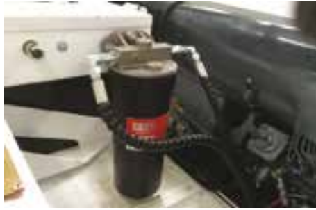
Bolted externally onto the machine is one of WearCheck's bypass filters for the transmission. The filters have already saved a mine over R1,5 million during an initial trial process.
