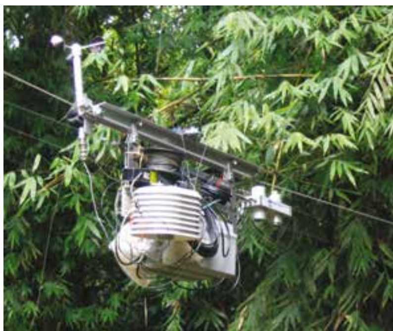
The NIMS measurement unit using CompactRIO and LabVIEW traverses on a cable between towers at the La Selva Biological Station.
