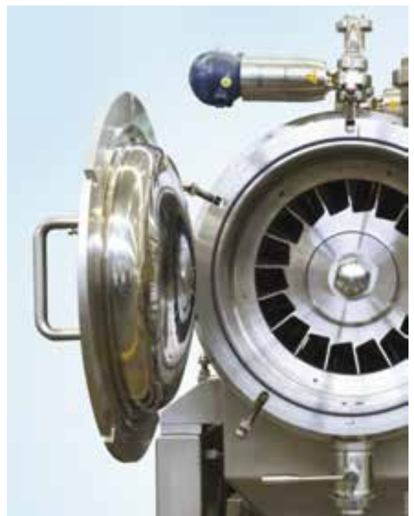
Figure 3: The Turbo Finisher is designed for puree production from chopped chunks of berry and other vegetables/fruit
