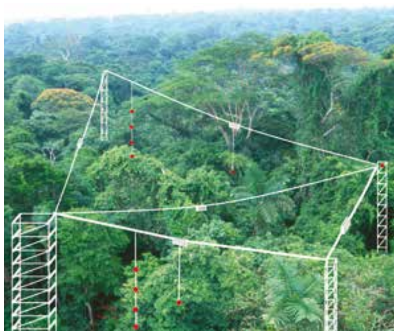
The NIMS based on NI technology will help researchers take better measurements at the La Selva Biological Station.
