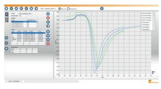
LayerSolver<sup>™</sup> is a dedicated software module that allows fitting of multiple nanolayers simultaneously from multiwavelength measurements.
