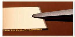
Choose a substrate. Use ready substrates including Au, Ag, Pt, Al, SiO2, TiO2, Al2O3, PS, PDMS, nanocellulose etc., or make your own using CVD, ALD, LB, sol-gel, spin coating, electrodeposition, self-assembly, or others.
