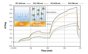
Real-time swelling of nanocellulose under different water vapour concentrations.
