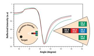
Even subnanometer differences in the inner and outer circles within a CVD chamber can be measured using MP-SPR. Here, MP-SPR discovered a 10 nm difference in metal deposition thickness towards center and 0.2 nm difference along the outer circle.
