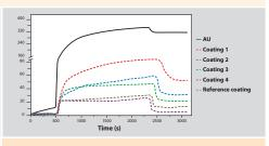
Measure interactions in real-time: adsorbed protein mass, release kinetics, swelling, etc. Here, a protein-resistant coating is evaluated.
