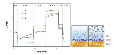
PAA polymer brushes swelling and collapse caused by pH and electric potential change.
