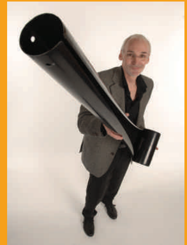
▲ RolaTube is a newly developed bi-stable reel composite (BRC) that can be repeatedly rolled and unrolled from flat spool to rigid tube
