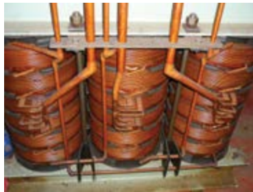
Figure 7: Bobbin type winding.
