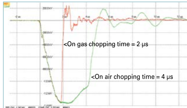
Figure 19: Comparison voltage - lightning impulse chopped on gas (1 350 kV) and chopped on air (1 705 kV).
