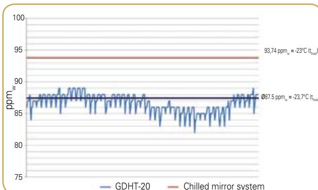
Figure 1: Comparative measurement between a chilled-mirror dew point meter and a GDHT over 24 hours on a switchgear system.
