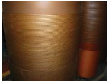
Figure 6: Cylindrical type winding.
