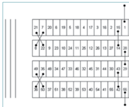
Figure 8: Model of the first discs of the interleaved winding of the transformer under study.
