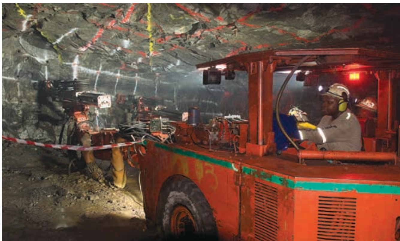
Below: A twin boom Sandvik rig at work in the UG2 North mine.
