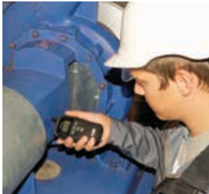
The entry-level VibChecker portable instrument, designed for reliable on-site vibration measurement and assessment.
