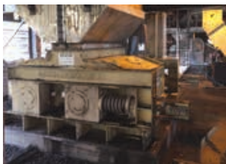
Osborn 3054 double roll crusher working at a coal operation near Lephale.
