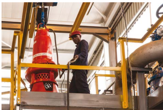
PIC 02: The first test run at Integrated Pump Technology's new 90 kW test tank facility, carried out on a Grindex Bravo 800 pump.
