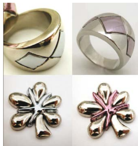
Figure 3: Bi-metal castings of micro-alloyed AuGa 2 blue gold (left) and micro-alloyed AuAl 2 purple gold (right) with 95 wt% palladium [9].
