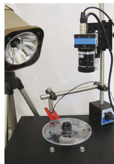
Figure 2: (a) Schematic of the components required for fluidic control and imaging of the disc device and (b) the integrated testing system set-up
