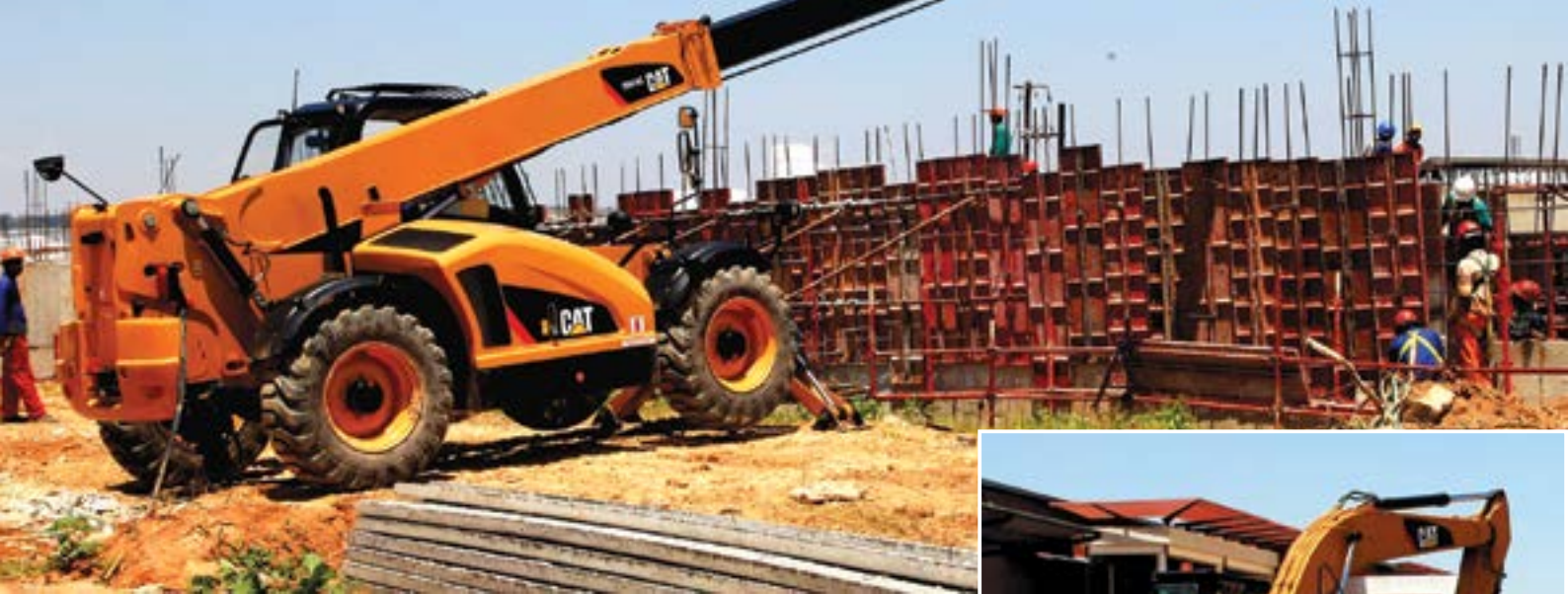
The Cat TH414C has a maximum lift height of 13,7 m and maximum forward reach of 9,2 m.
