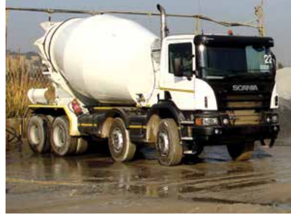
Scania's two models offer 310 and 410 hp respectively. The P310 generates 228 kW and the P410 302 kW.
