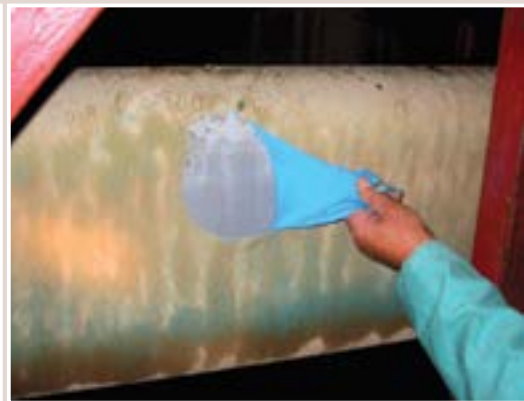
ABOVE, LEFT: Filter Focus COO Craig FitzGerald. ABOVE, RIGHT: Rust-Prufe is environmentally-friendly and with zero toxicity leftover, the coating can be disposed of safely in landfills. RIGHT: Upon application, the product is peeled off by hand to reveal a clean and rust-free surface.
