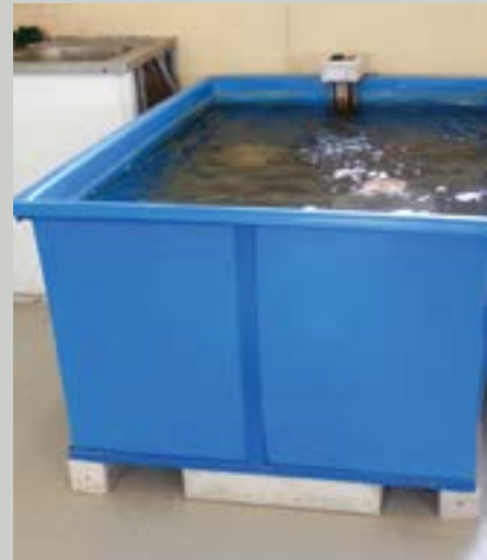
The curing baths at the Concrete Centre of Excellence.
