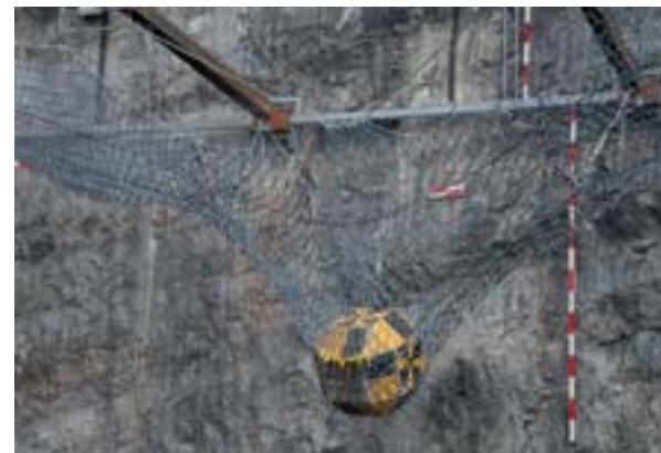
A Geobrigg ring net stopped a 20 tons concrete cube with an impact velocity of 90 km/h.
