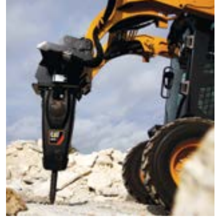
Cat skid steer equipped with the new Cat H55Es. The impact frequency (blows per minute) is 600 – 1 680.
