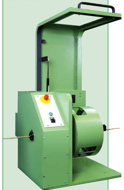
▲ Suitable for binding strand bundles with polyester yarn
