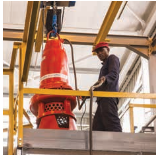
The first test run at Integrated Pump Technology’s new 90 kW test tank facility, carried out on a Grindex Bravo 800 pump.
