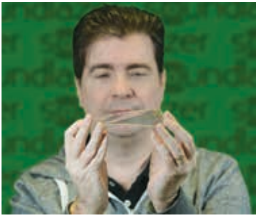
Kickstarter specialist Richard Haberkern demonstrates PVDF, a thin plastic polymer sheet with converse piezoelectric properties that make it ideal for use in audio speakers.
