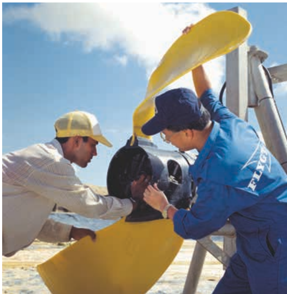
Above: Xylem SA offers full service support, via the local Total Care and mobile servicing offerings. Left: Xylem's signature Flygt 'banana blade' propeller has a large diameter and a backswept self-cleaning design for non-clog performance.
