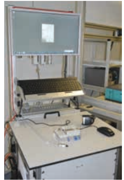
Each terminal block is automatically tested and certificated before leaving the facility.
