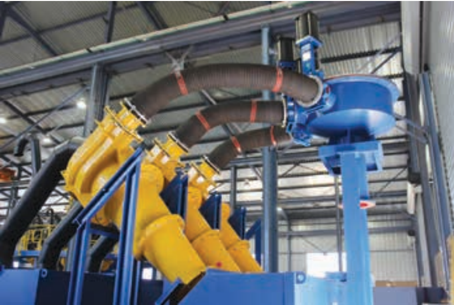
Above: Assembly of a 750 rubber-lined mill circuit pump at the Weir heavy bay foundry.
