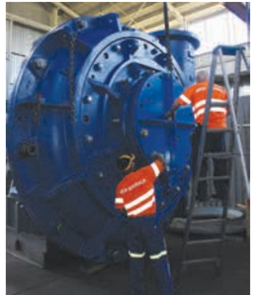
Above: Assembly of a 750 rubber-lined mill circuit pump at the Weir heavy bay foundry.
