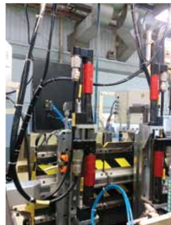
SMC's LEF actuators installed as preferred alternative to a bulky robot.
