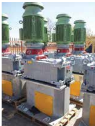
The acid mine drainage plant consists of a combination of 53 specialised Mixtec mixers.
