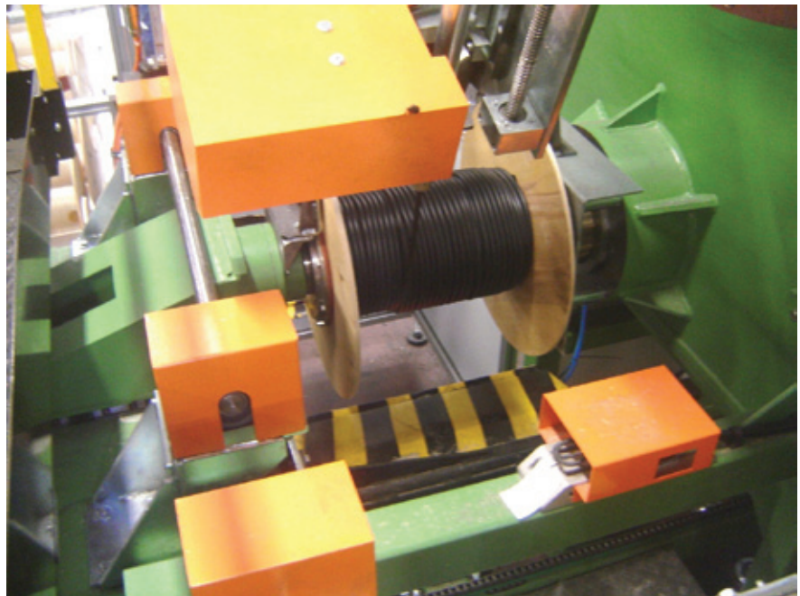
▲ The spooling phase in the new PS630/15 2B
