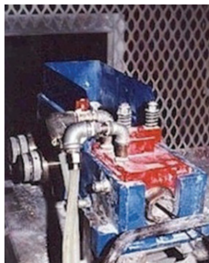
▲ Rod coating and lubrication by LVC/PDH system
