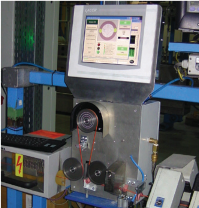
○ Figure 10: Prototype of Siebe colour measurement system during test at a customer's line. Installation between spark test and lump camera. IPC at the top, below, turn mechanics and sensor (under light cover)
