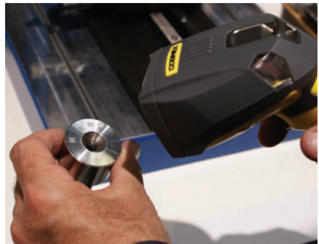
▲ Identification of an EDDS-2 marked die-tool
