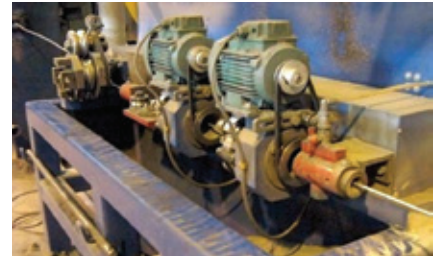
▲ Rod cleaning and wire drawing by DCCD process
