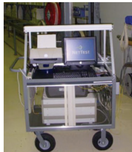
▲ Figure 5: Optical fibre strain gauge measurement system
