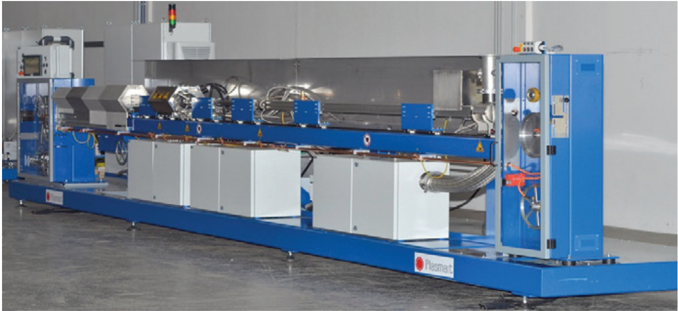
▲ Plasma Annealer for high speed annealing of stainless steel and nickel alloy wire
