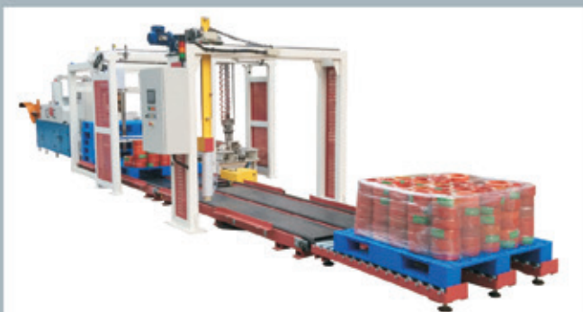
Auto coiling and stacking line
