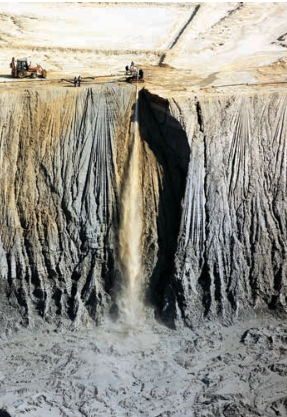
DRDGOLD's dump retreatment operation is a high volume, mechanised business which primarily makes use of high-pressure water jets.
