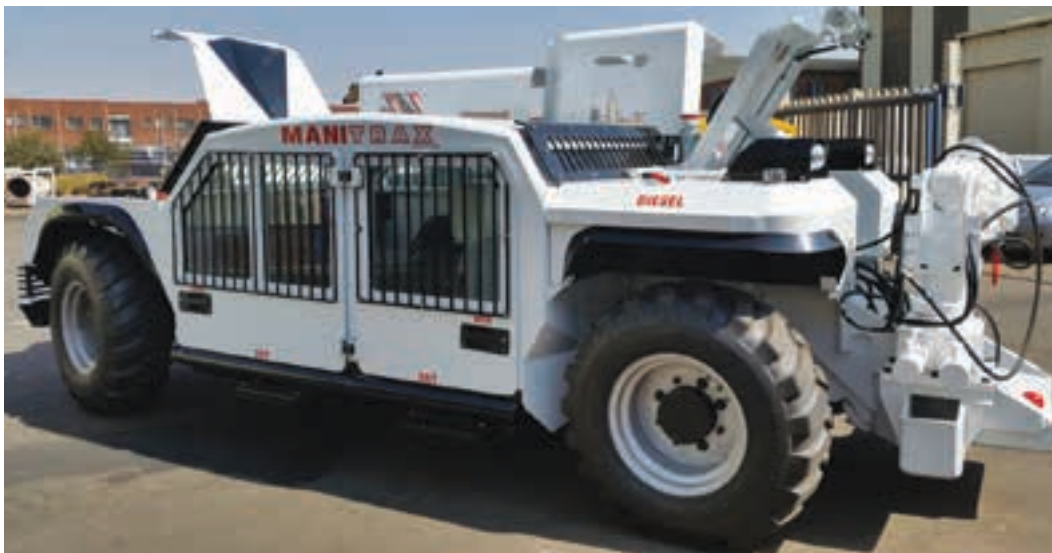
The Manitou ManiTrax 35-ton tow tractor is designed for underground and confined spaces. It has received various modifications since it was unveiled at EMA 2014.
