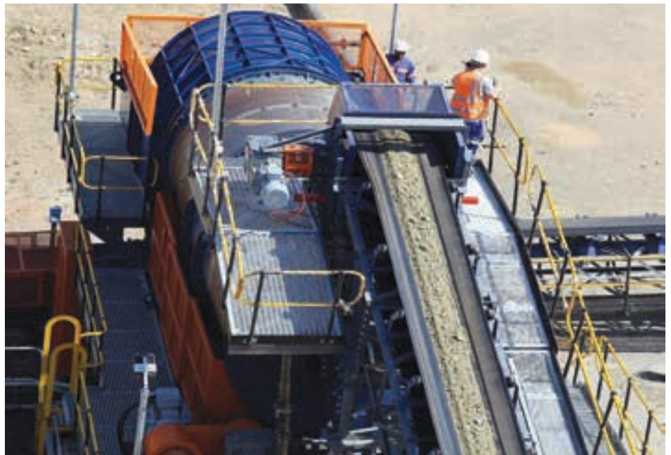
Kimberlite ore from the primary crusher at Lerala being fed into the new primary scrubber (photo: Kimberley Diamonds).
