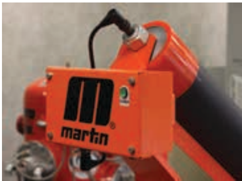
The Martin® Roll Gen™ system is a self-contained mini power station.
