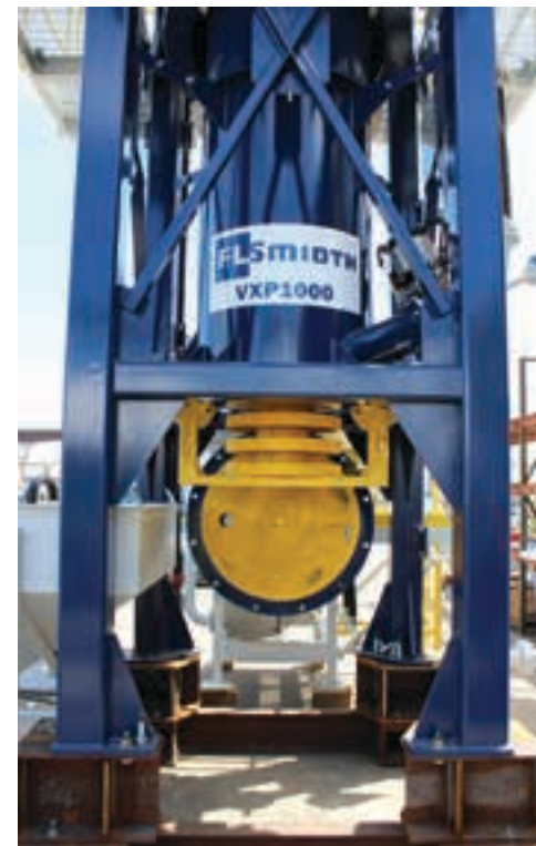
Disc maintenance on the VXP1000 can be done safely from below the grinding chamber.
