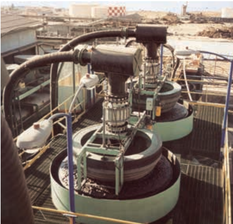
Pneuflot® cells are simple in design, with a high yield of froth product.
