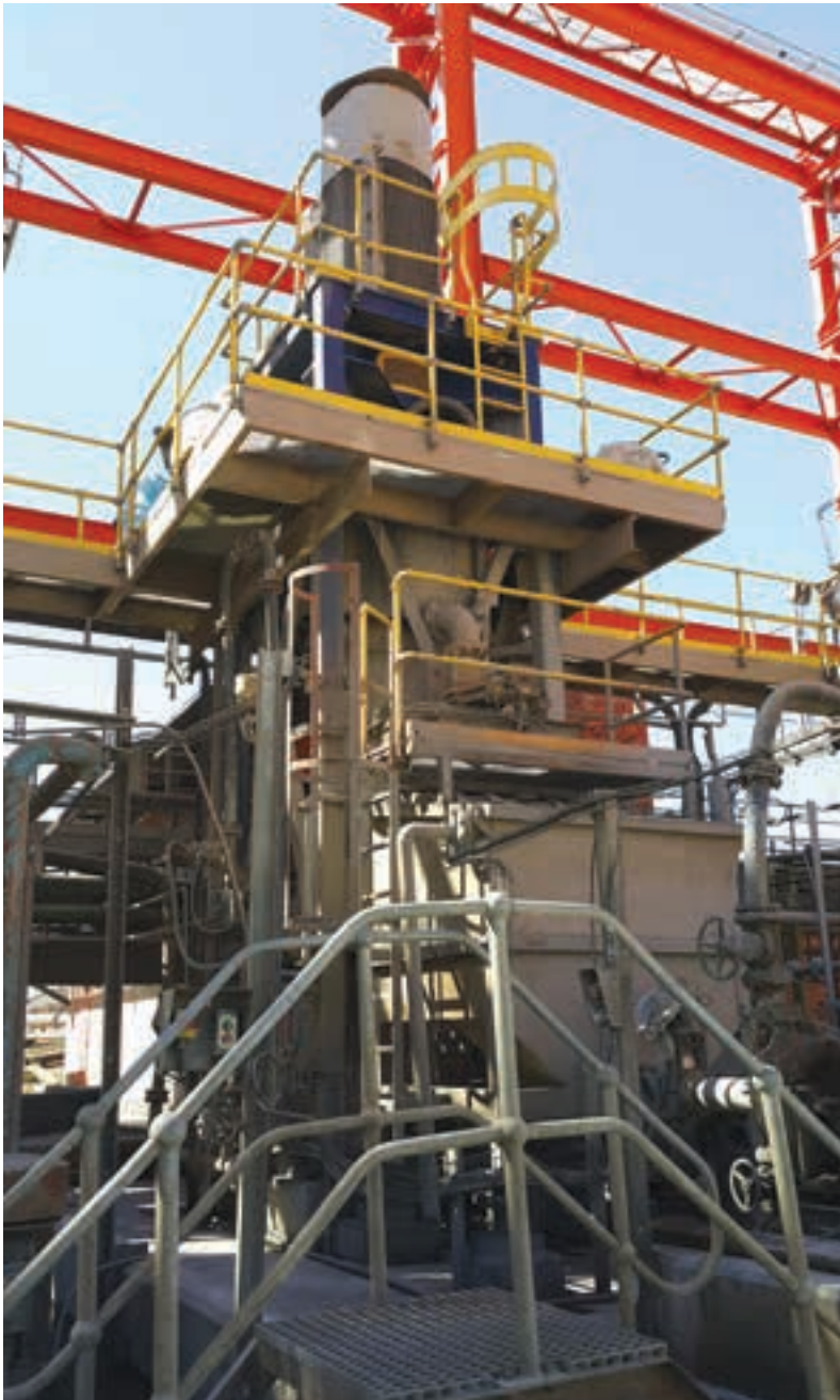
Above: One of the vertical mills in the fine grind section of the FFG circuit (photo: Arthur Tassell).
