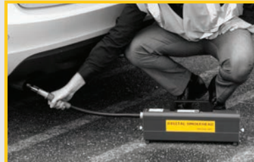
Digital smoke meter with automatic calibration
