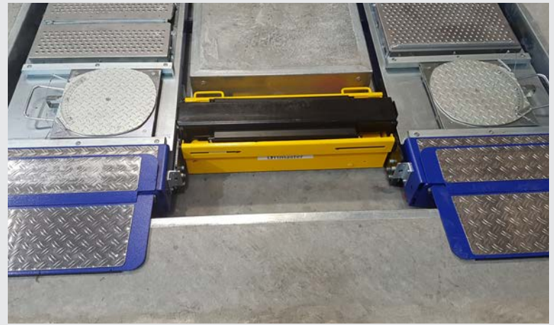
Sunken Jacking Beam
