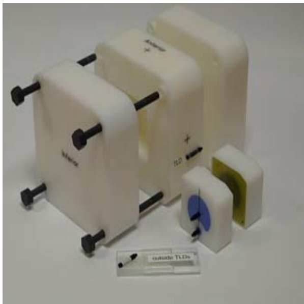
Fig. 1 IMRT phantom with an insert loaded with film and TLDs.
