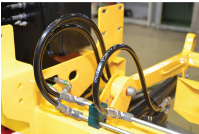
Hydraulic installation on an MBB-Palfinger lifting platform: interaction of tubes with Voss cutting rings and couplings as well as hoses Image copyright MBB Palfinger GmbH
