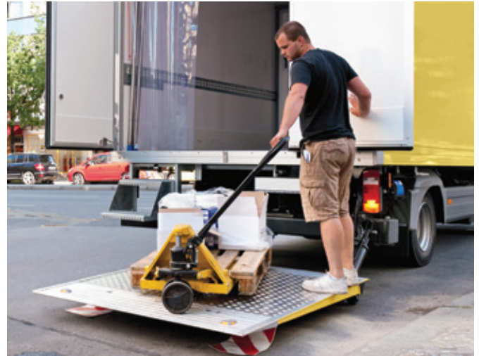
Application example: small truck with lifting platform Image copyright MBB Palfinger GmbH
