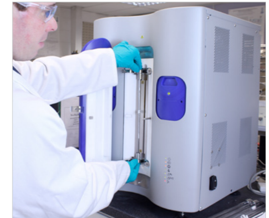
iGC-SEA straight column design - simple sample packing and column loading
