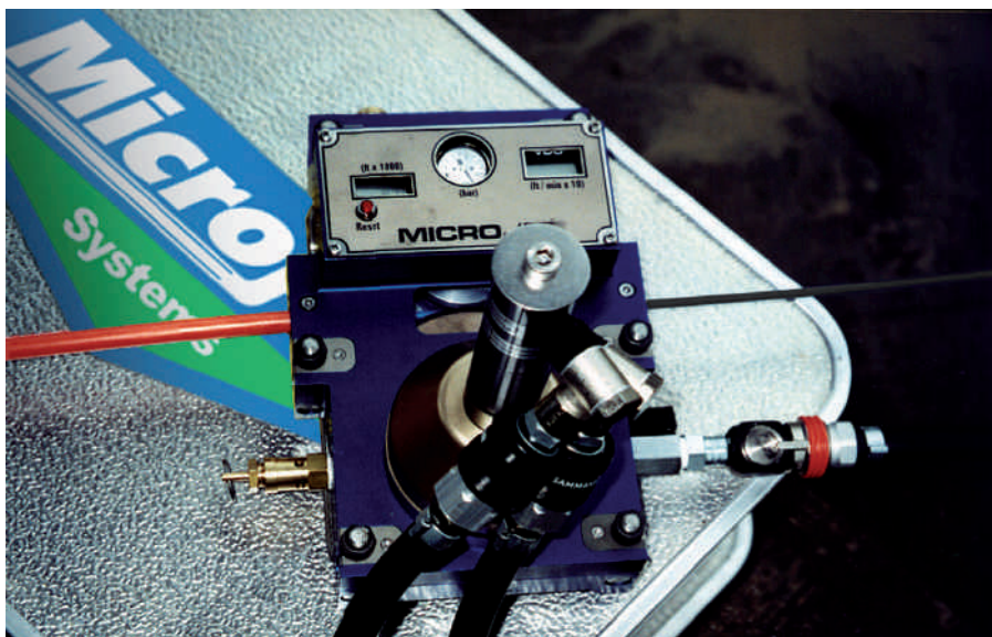
▲ Figure 12: Micro cable blowing
