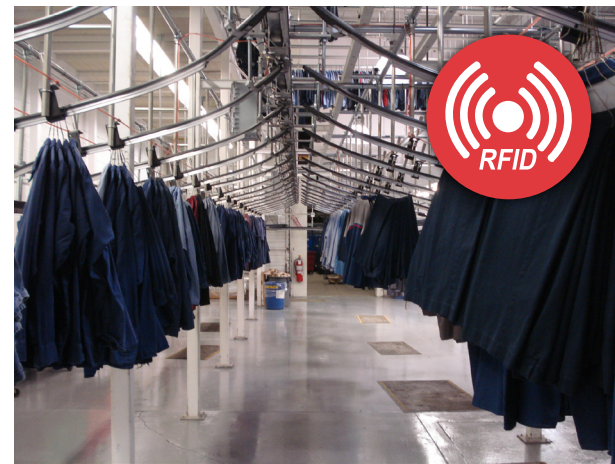
Garments are automatically sorted by wearer and ready for final scan at checkout.
