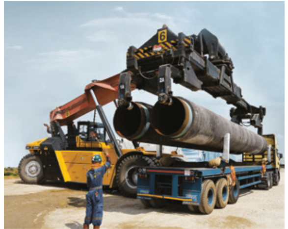
Concrete weight coated pipes
