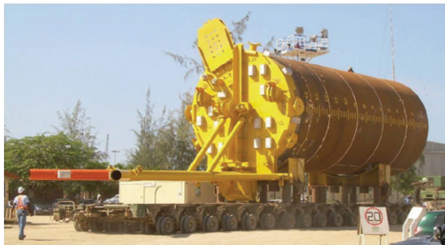
A typical 100t pipeline suction anchor, installed on Greater Plutonio field, offshore Angola Photo credit: Jayson et al – Offshore Pipeline Technology Conference 2008
