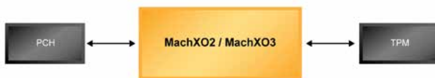
Fig. 8: LPC to SPI Bridge for TPM.
