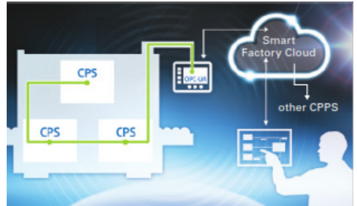
Figure 2: Several autonomous Cyber Physical Systems (CPS) are vertically integrated into a Cyber Physical Production System (CPPS) that is connected to the Smart Factory Cloud and controlled by a Smart Factory Manager
