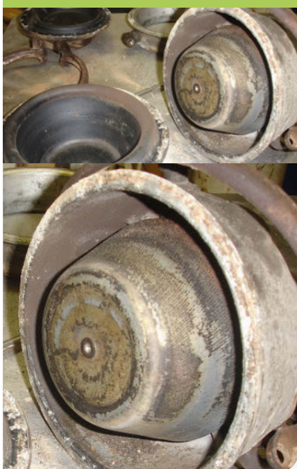
Excessive corrosion inside the brake chamber
