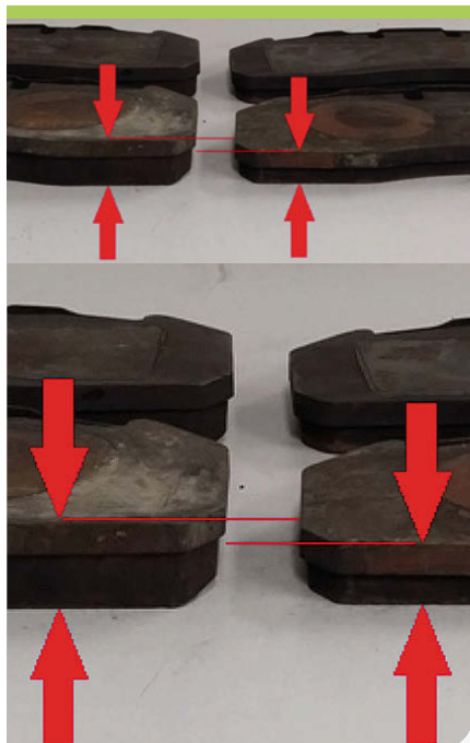
Thickness difference between calipers of the same axle
