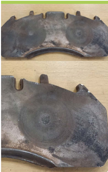
Damaged brake pads due to incorrect fitting or application
