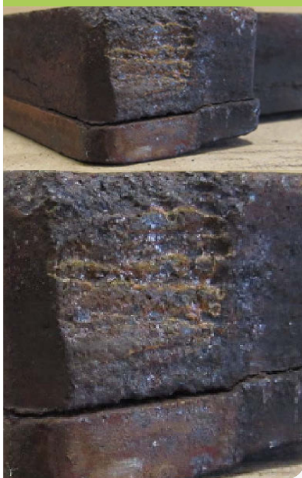
Damage on brake pad's seats and friction material
