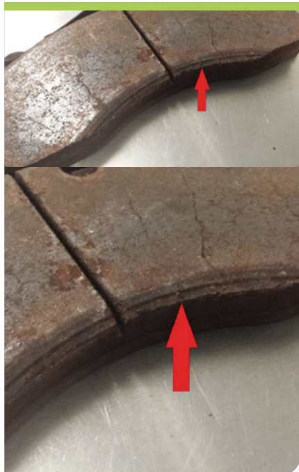
Uneven wear-lip groove on inner and/or outer radius
