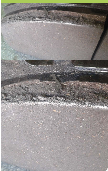
Localized crumbling of the friction material
