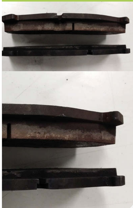
Thickness difference between inner & outer Caliper's pad
