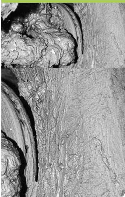
Extreme brake wear due to off-road use
