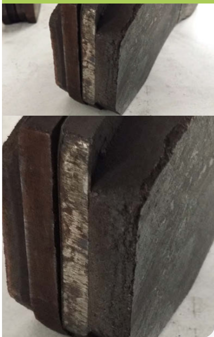
Brake pads are dimensionally modified (grinded)
