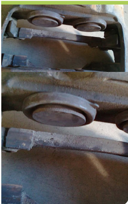
Pistons' rubber boots and other sealings are scorched
