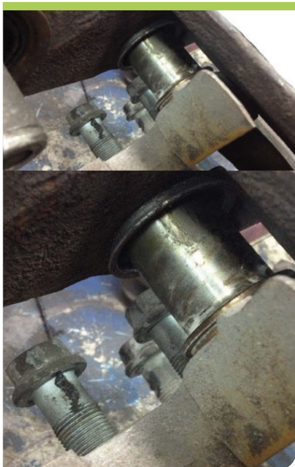
Caliper's guide pins & bushings require maintenance
