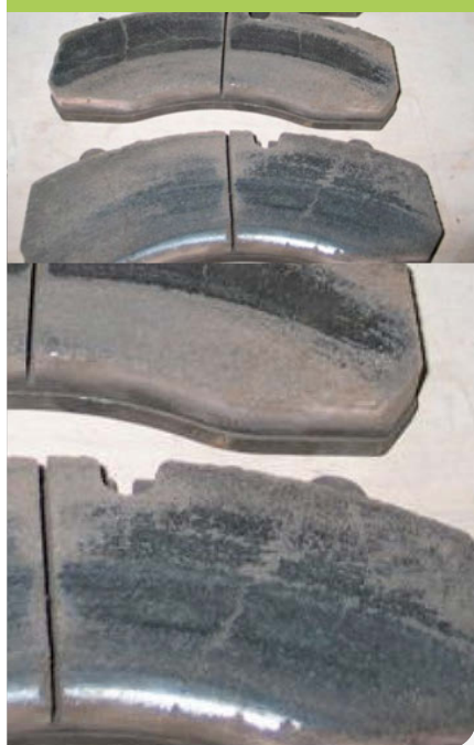
Brake pad's friction surface is glazed
