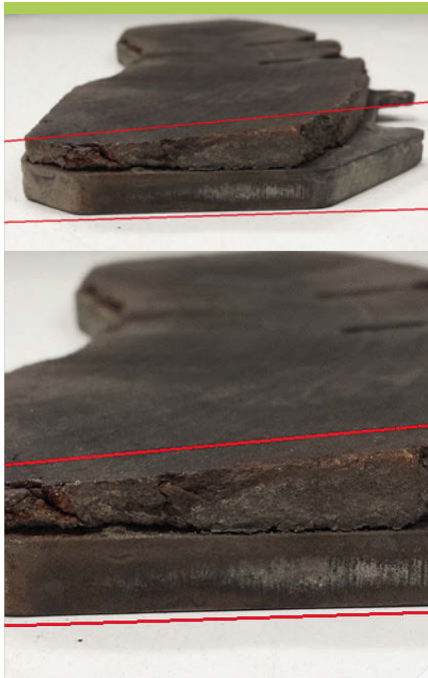
Angular wear on the same brake pad (x, y or x & y axis)
