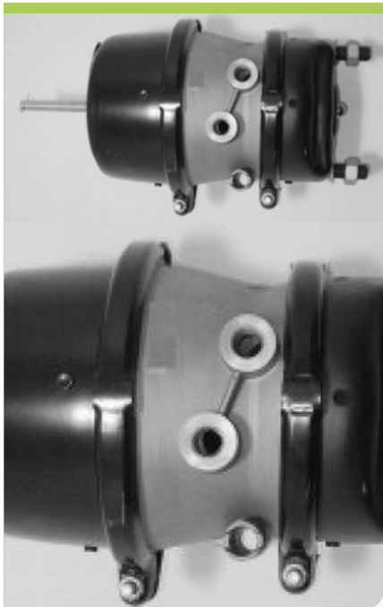
Air leakage in the area of diaphragm or clamping band
