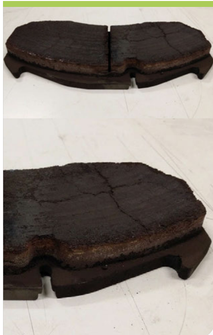
Friction material has cracks, rusty look and/or white edges
