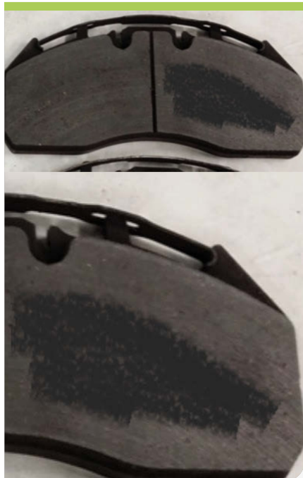
Friction surface is contaminated with oil, grease etc.
