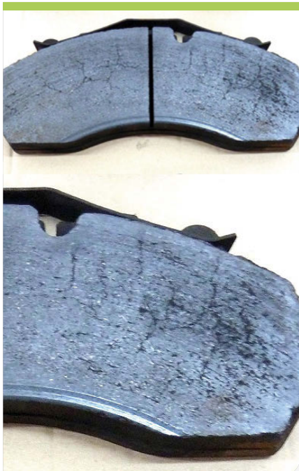
Small cracks on the friction surface
