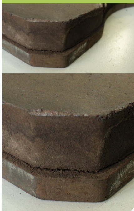
Partial or full separation due to high thermal stress
