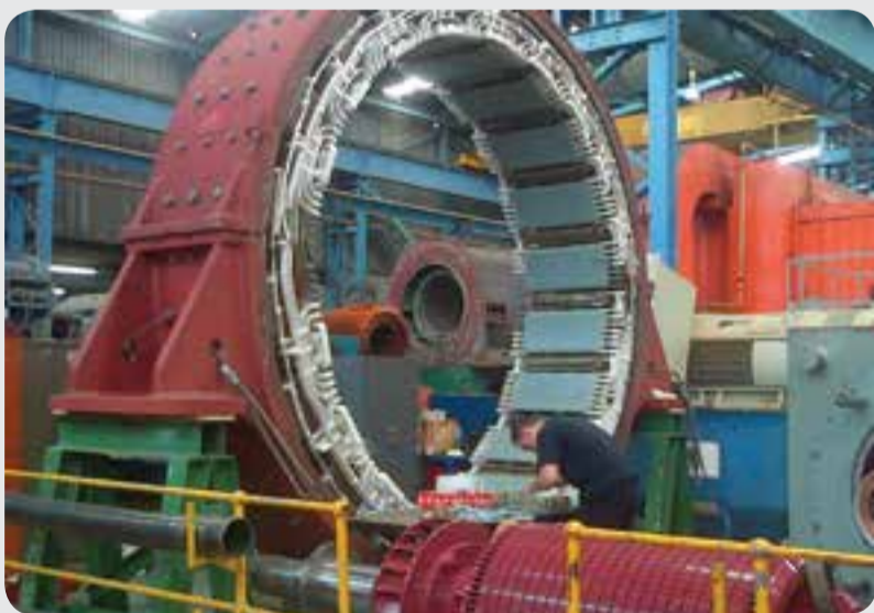
Jarred van den Bergh, an apprentice at Marthinusen & Coutts, laying out the insulation tapes for the winders in order to complete final taping on the field frame leads.
