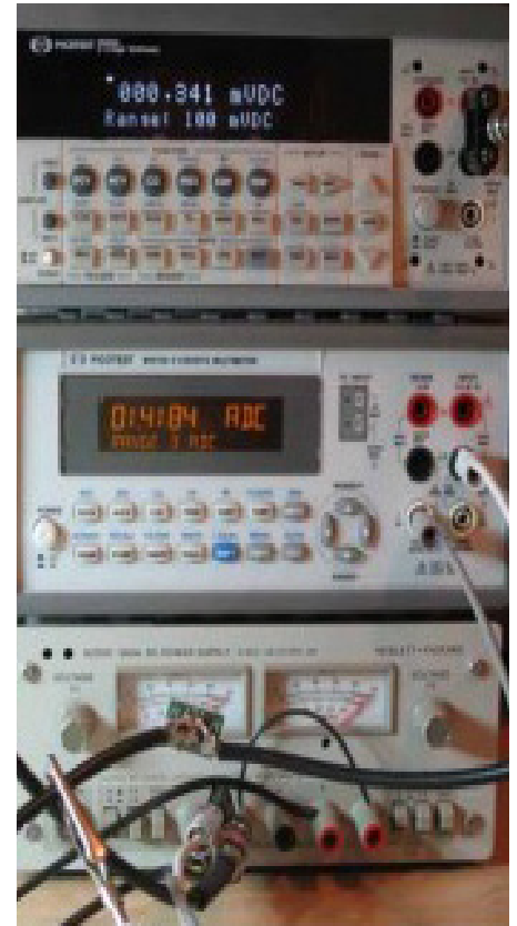
Figure 5 A DC measurement is made using precision, low noise 6.5 Digit DMMs (Picotest M3500A) to obtain a second measurement for correlation. The power supply does not have current programming, which is the reason the current is set to an odd number. The two channels of the power supply are connected in parallel and both are in current limit for this measurement.
