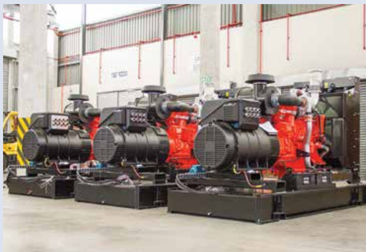
The three 450 kVA generator sets for the Silo 3, 4 and 5 Project prior to testing at the Zest WEG Group Generator Sets facility in Cape Town.
