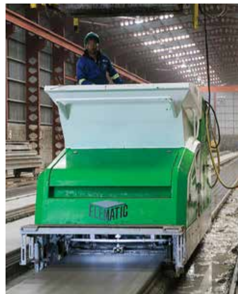
Hollow core slab production.
