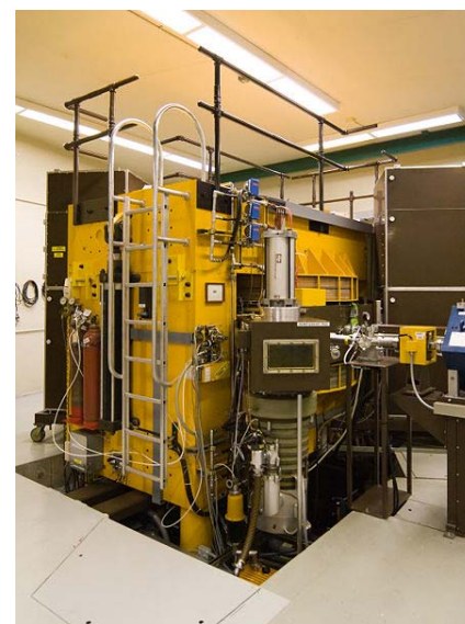
Cyclotron for production of diagnostic radionuclides
