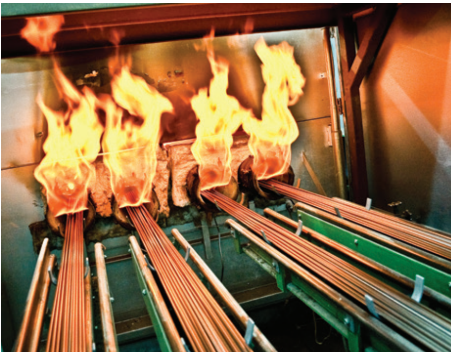
Stainless steel tubes on their way to the heat treatment section
