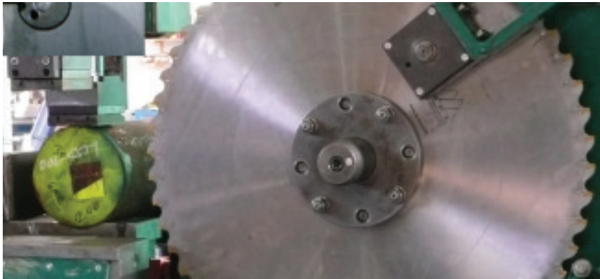
MFL's sawblades feature exchangeable carbide tips
