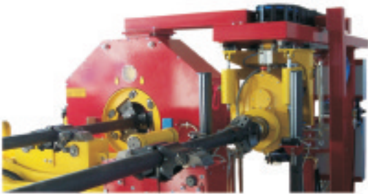
Fig. shows a 7" / 18 kft-lbs machine with open style backup and on the right side mounted external pre-tightening station.
