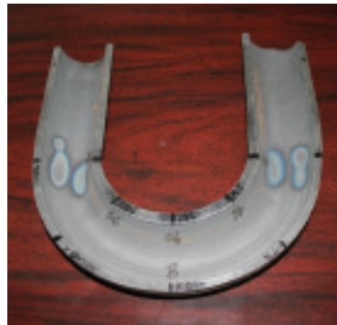
Photo 4: Cross section of sample No. 8 showing the outer and inner walls of the tube bend
