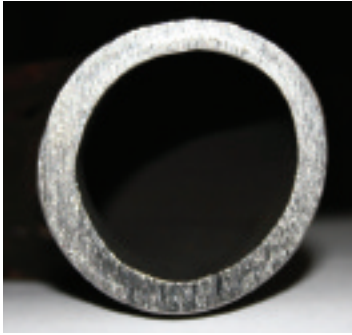
Photo 5: Cross section of sample 12 at the bend location of 45° showing the outer wall thinning, the inner wall thickening, and a small amount of ovaling
