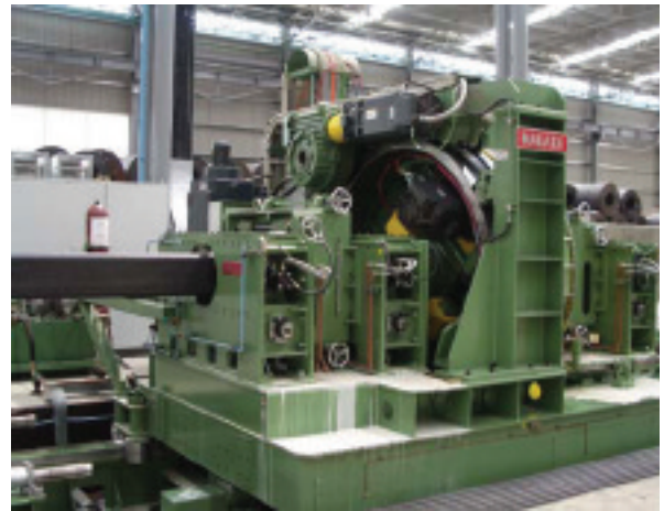
12" Milling type flying cutoff machine
