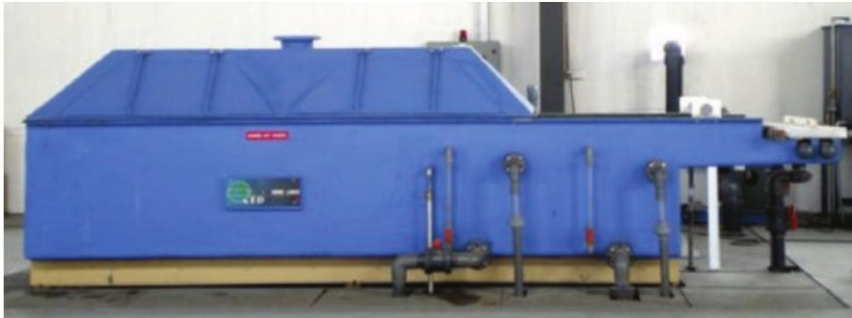
▲ QED Wire Lines' pre-clean system
