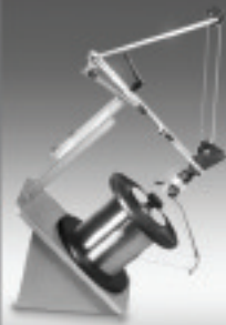
Payoff with dancer accumulator and double pivot to pre-load
