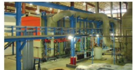
▲ Cleaning and descaling of carbon and stainless steel wire and rod
