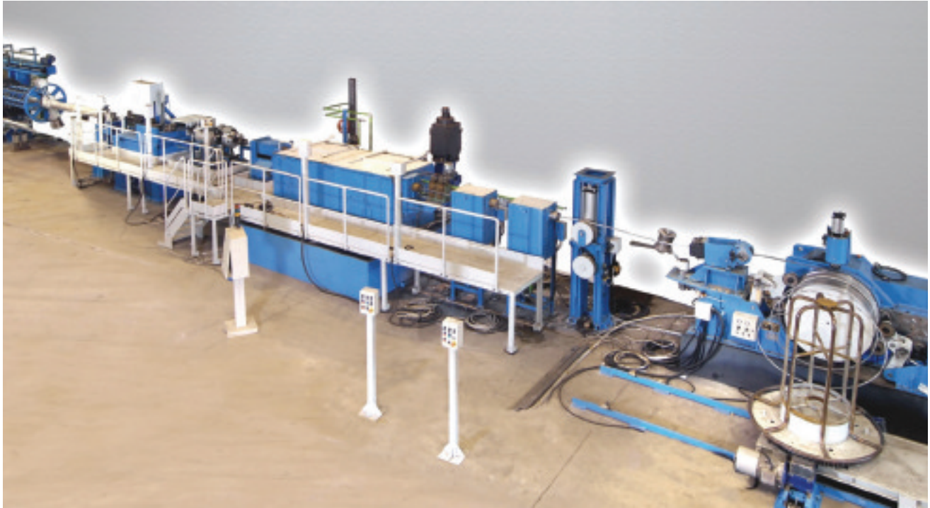
▲ Typical wire cleaning line from ICMI
