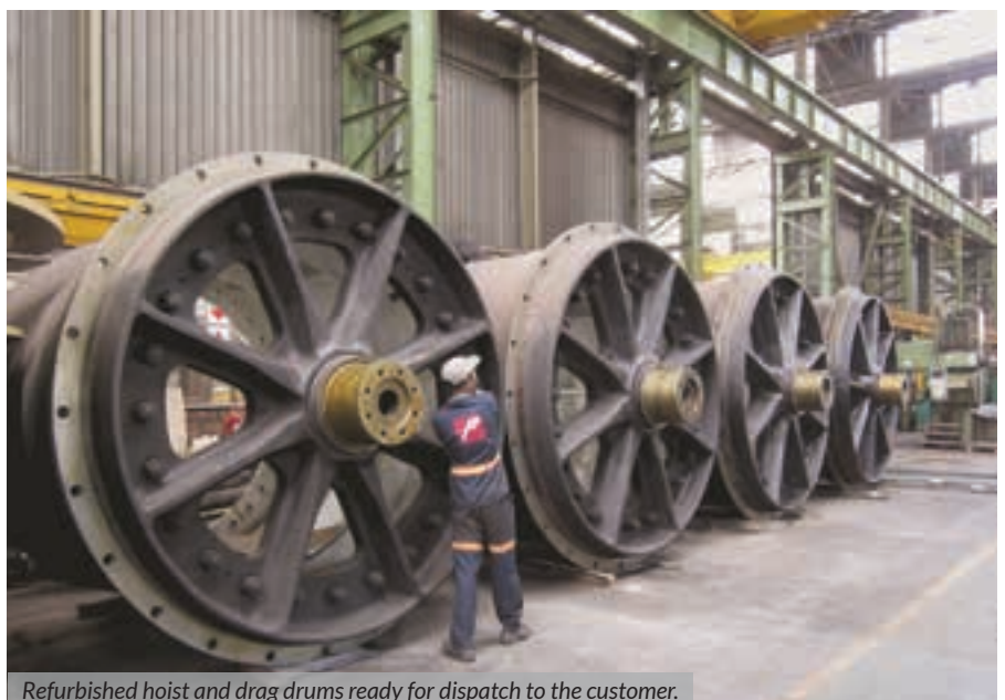
Refurbished hoist and drag drums ready for dispatch to the customer.
