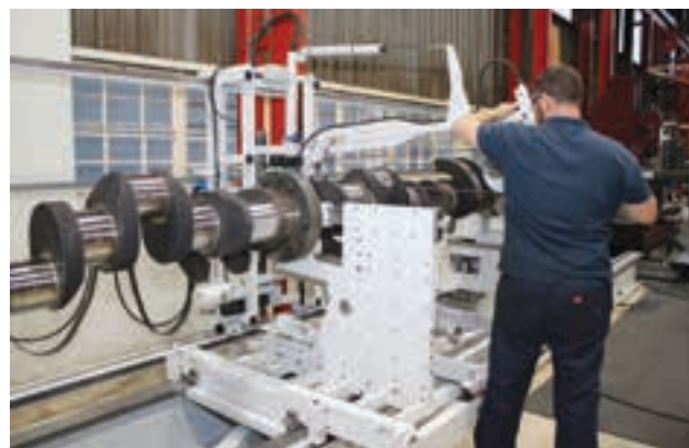
Metric Automotive Engineering's custom engineered, one-of-a-kind crankshaft polishing machine is capable of accommodating crankshafts with lengths of over six metres.
