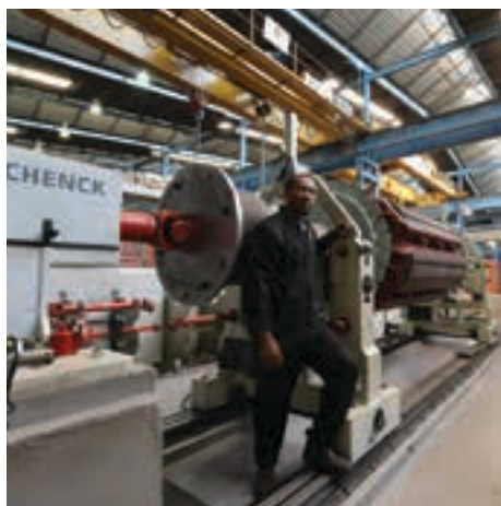
The 32 t Schenck HM7 U/S balancing machine, at Marthinusen & Coutts' 9 500 m 2 workshop.
