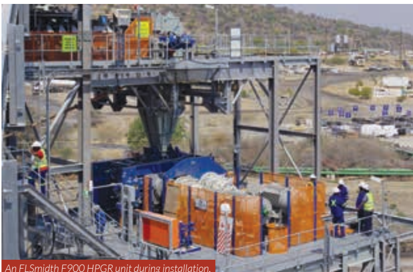
An FLSmidth F900 HPGR unit during installation.
